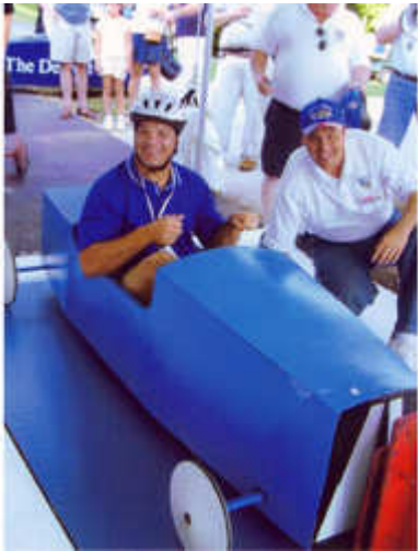
The American Corporate SBD car. Built of plywood it uses Super Stock car standard running gear
