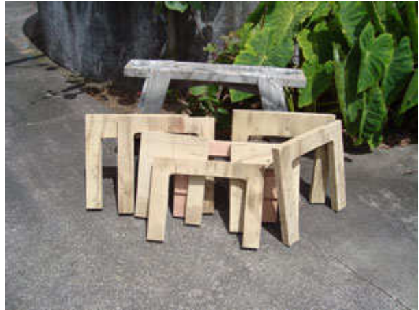
The ribs – ply laminated, screwed together and ready for shaping
